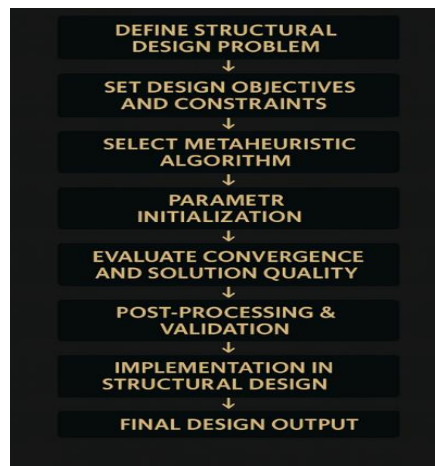
Figure 1: Workflow for structural design optimization using metaheuristic algorithms
